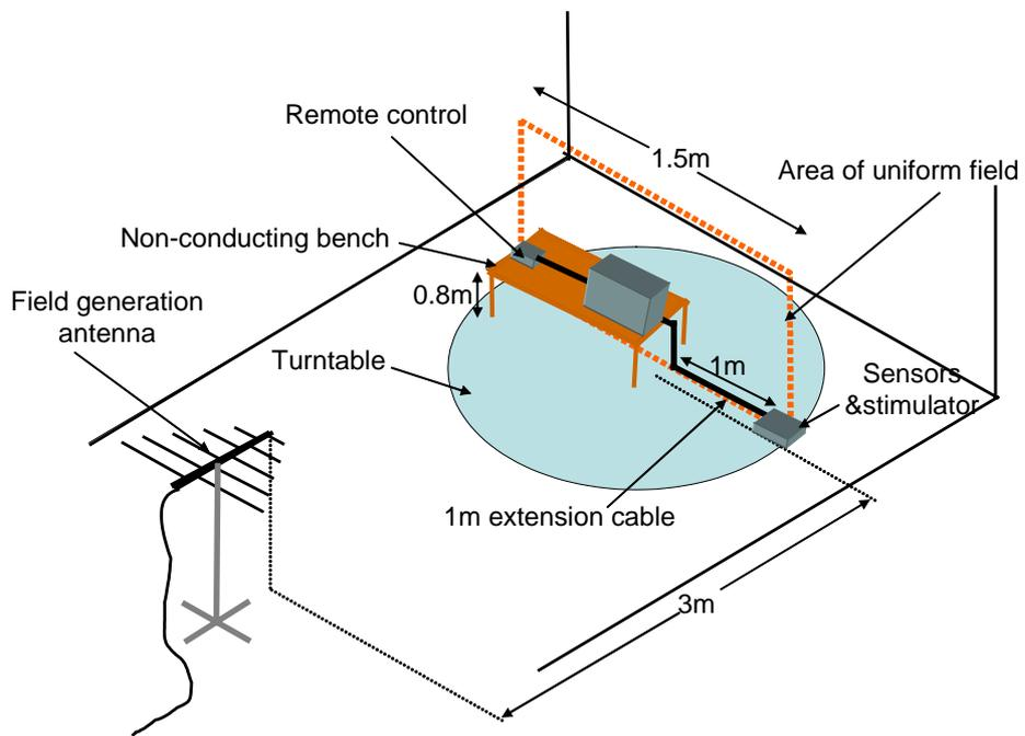
FIGURE 2: Plan view of a typical EMC test layout
